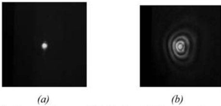
Fig. 8. He-Ne probe beam profile (a) when 1.55 \mu\text{m} pump beam is off (b) pump beam on. A118 dye-doped 5CB film.
